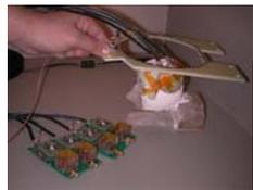
The arrays consists of 3cm diameter actively detuned coil elements cut on a CAD controlled circuit board milling machine. The array is shown over the monkey head model made from MR data and 3D printing methods to aid in the construction of custom fitted helmets for the individual monkeys used in the fMRI experiments.
