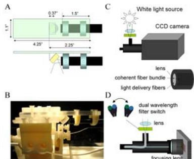
**Figure 2. MR-compatible optical imager.** A. The distal end of the fiber bundle is coupled to a mirror (yellow). B. A photograph of the distal end mounted onto the animal holder. C-D. At the proximal end the imaging fibers in the bundle are coupled to a CCD detector. Light from the light source is passed through a dual wavelength filter switch and focused onto illuminating fibers.
