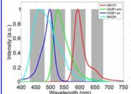
**Figure 2. Emission spectra and filters.** Emission spectra of NADH (cyan), OGB1 (green) and SR101 (red) are shown in relation to bandpass filters used for the measurements (gray rectangles). The excitation spectrum of OGB1 (1-photon excitation spectrum is shown in blue) significantly overlaps with NADH. As a result, OGB1 absorbs NADH fluorescence preventing simultaneous imaging.
